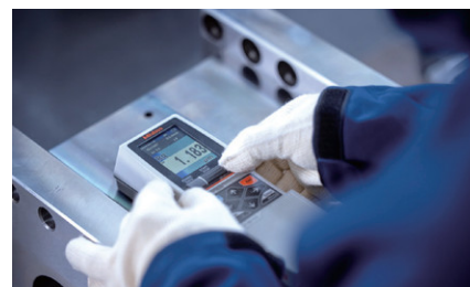
Roughness tester measures roughness of extruder barrels
