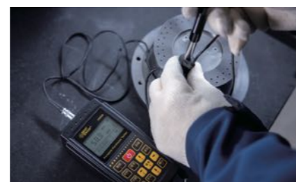
Leeb hardness tester measures the hardness of extruder components
