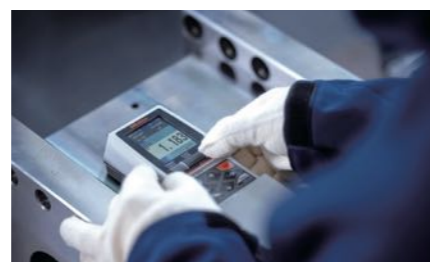
Roughness tester measures roughness of extruder barrels
