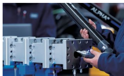
Three-coordinate measuring machine measures overall coaxiality
