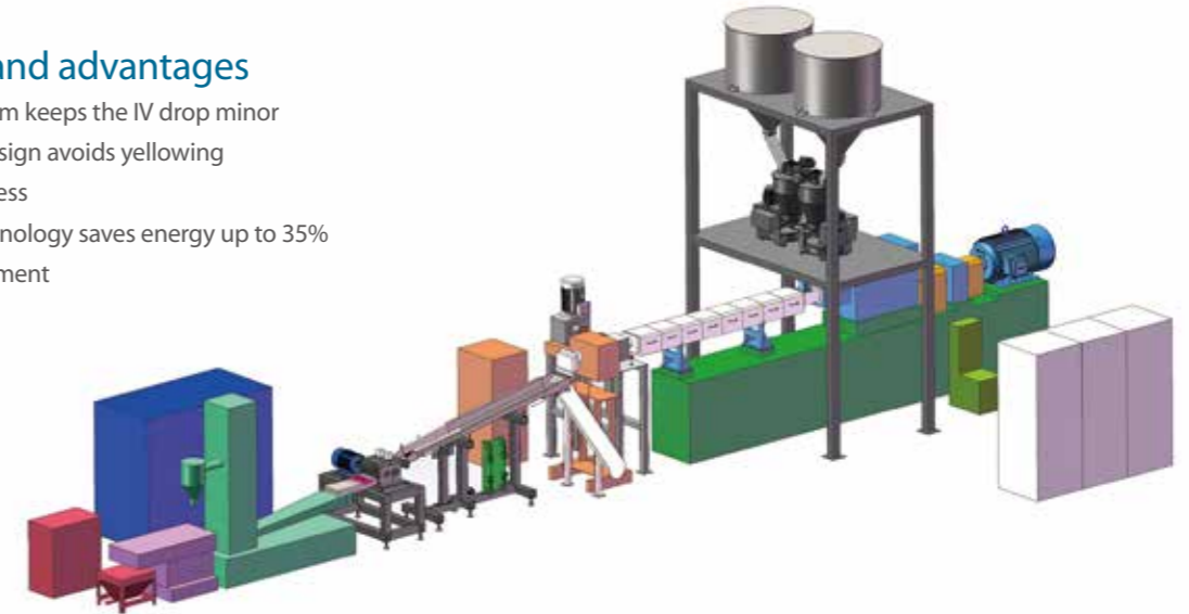
PET bottle flakes recycling and pelletizing line
